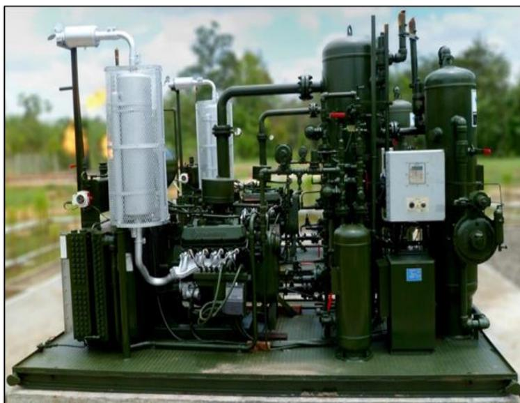
**Figure 1** Gas jack compressor (Compressco, 2009)
